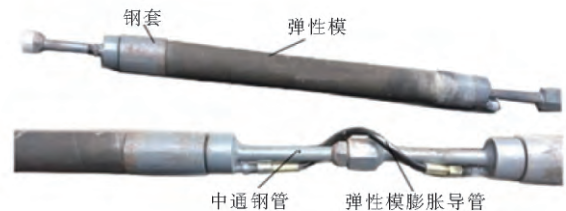
图 5 跨式膨胀型封隔器封孔示意图 Fig. 5 Diagram of sealing with straddle expansion packer
